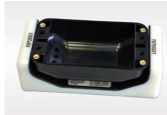
Figure 6: Injection molded part (black) with heat-staked brass inserts rests in a PolyJet multi-material fixture (VeroWhite and TangoBlack).
