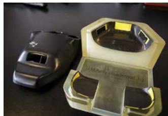
Figure 3: Assembly fixture (right) has non-marring, anti-slip (black) interface surfaces (FC720 and TangoBlack™).
