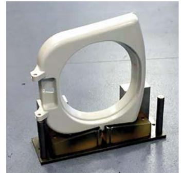
Figure 7: Assembly fixture printed with rigid and rubbery features (FC720 and TangoBlack).
