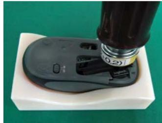
Figure 2: Computer mouse (black) and assembly fixture (white) for inserting screws (VeroWhite™).
