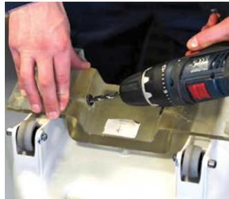
Figure 1: Printed drill guide (FC720).
