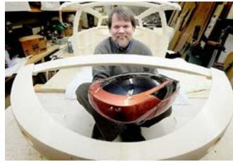
Jim Kor with the Urbee prototype and FDM full-scale, functional body panels bonded.
