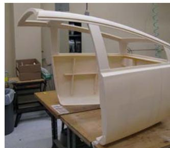
One benefit of bonding FDM parts is the ability to section fine features and build them with a finer slice setting, allowing for a more accurate part.
