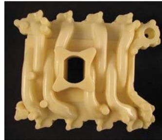
FDM manifold for functional testing.
