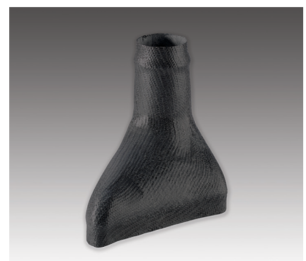
Figure 3: The FDM tool is easily removed, hands free, leaving the final composite part.
